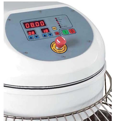
Fitted with 2 independent motors, both reversible: one to turn the bowl plus a 2-speed one for the spiral.
