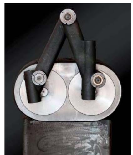
The arm shafts are made of F-155 steel, for maximum protection against the twisting forces which come about.
