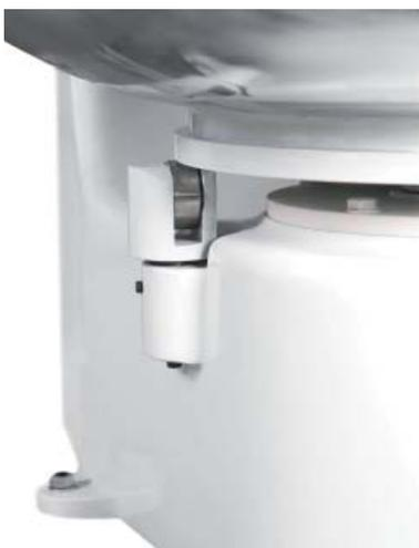
The bowl support plate with side support wheel eliminates any swinging, increasing the useful life of the machine and its components.
