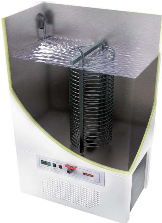
It is fitted with electronic control and an shaker to ensure exact, uniform water temperature. The vat is made of AISI 304 stainless steel for maximum protection against corrosion. Insulated with injected polyurethane sandwich panels to minimize energy loss. Capable of reducing the temperature of 175 litres of water by 5°/hour with consumption of just 0.45 kW.
