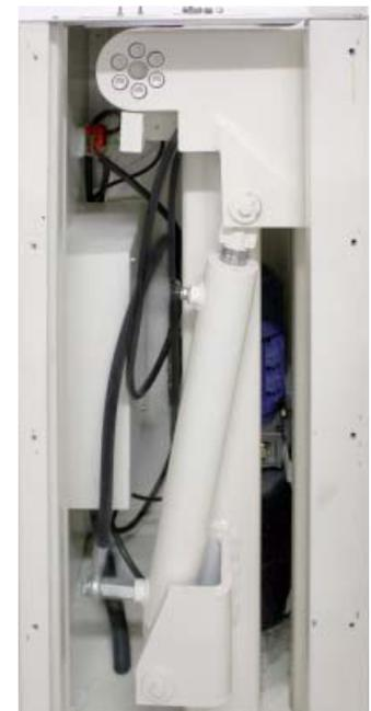
The elevation system comprises 1 hydraulic piston, which tips the mixer on the table.
